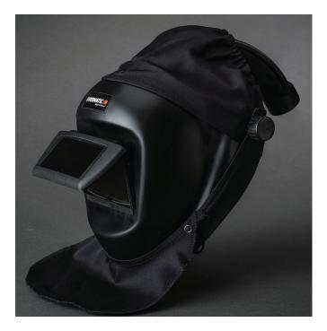
Evermatic Air is a lightweight welding helmet with respiratory protection for professional use. It comes fully assembled, complete with fabric covers and an air duct. Positive pressure maintained inside the helmet prevents harmful particles from entering the breathing zone. The helmet protects the wearer against particulates, such as solid and liquid aerosols, welding fumes, and dust. Evermatic Air is based on the Evermatic welding helmet. Can be combined with hearing protectors.
